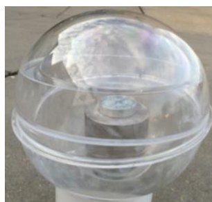
Figure 1: Two gravity-controlled N42 magnets in stack and deployment of one 135-pound smart rock in Roubidoux Creek, Missouri.
